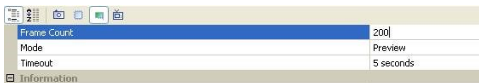
Figure 9-4 Frame count in the circular buffer for frame grabbing by the CL grabber card
