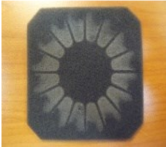
Figure 7-1 Dust on filter in front of the cooling fan
